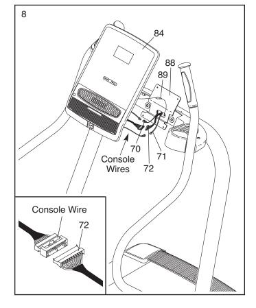
Attach the Console (84) to the plate on the Yoke (88) with four #8 x 3/4" Screws (1). Be careful not to pinch any wires. Start all four Screws before tightening any of them. Do not overtighten the Screws.
